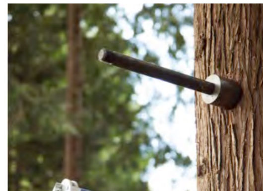
TAB installed in tree
