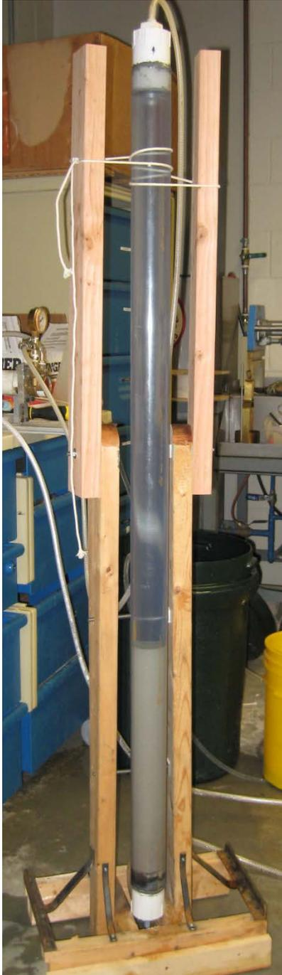
**Figure 1.** Sand Filter Apparatus
