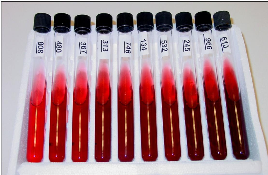
Figure 2 – Sensory analysis experimental setup to rank color visually by a panel (n≈70)
