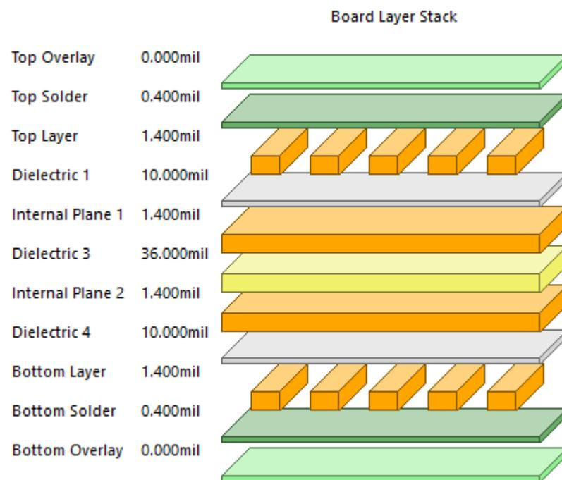
Figure 4. PCB Layer Stack
