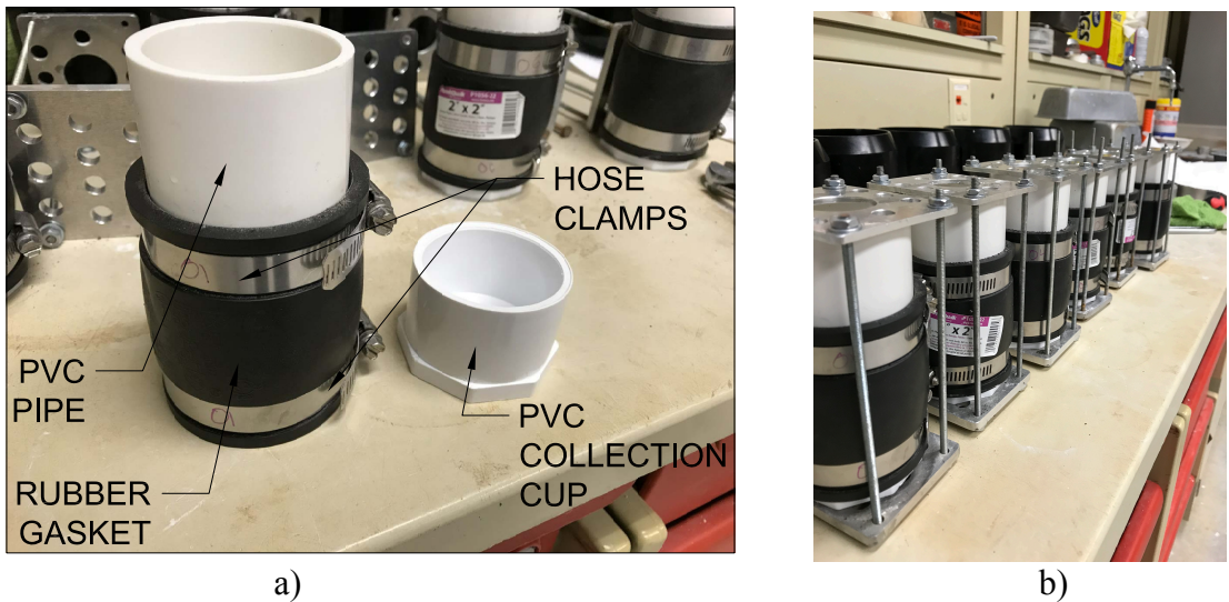
Figure 4. a) A soil testing apparatus and b) each soil testing apparatus in the respective aluminum cage prior to placement into the sampling bucket.
