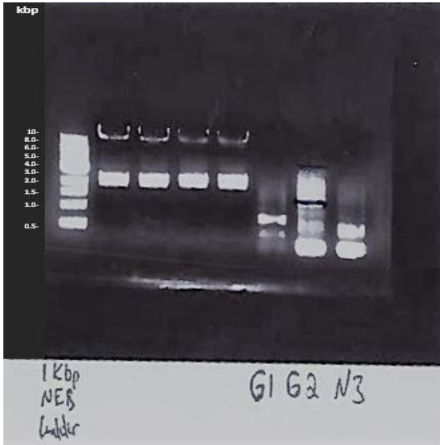
Figure 5: Seventh Polymerase Chain Reaction (PCR) Experiment on 0.5% SDS Gel with 1Kbp NEB Ladder, Primers CcmFUSGibFW & \sigma NB302 Product (G1), Primers CcmFUSGibFW & CcmFDSRV Product (G2), and Primers CcmFUSFW & CcmFDSRV Product (N3)
