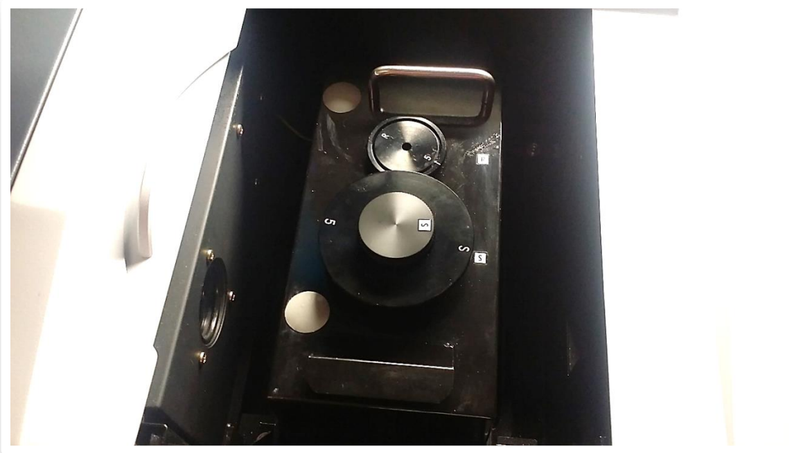
Figure 9. Shimadzu UV-3600 Reflectance Setup.
