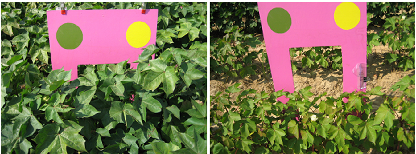
Fig. 1. Field off-nadir images of plots receiving 150 lb N/acre (LEFT) and 0 lb N/acre (RIGHT) with standardized color board in the background. Standardized color board consists of a dark green and yellow color chip on a neutral pink background to allow the normalization of each image during analysis. The high N rate treatment was taller and visibly darker green than 0 lb N/acre treatment.
