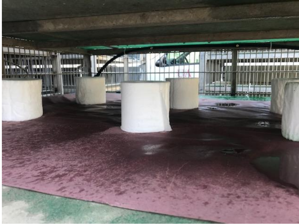
Figure 10: Cage floor after two spray cycles with significant pooling.
