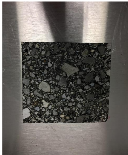
Figure 6. Specimen for Thickness and Squareness Tests
