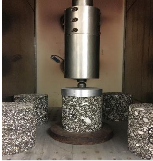
Figure 3. Equipment of compressive strength test
