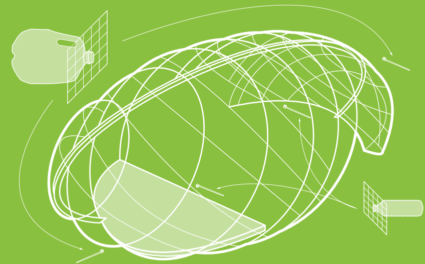
Secure the mesh panels with the bottles to the structural frame
