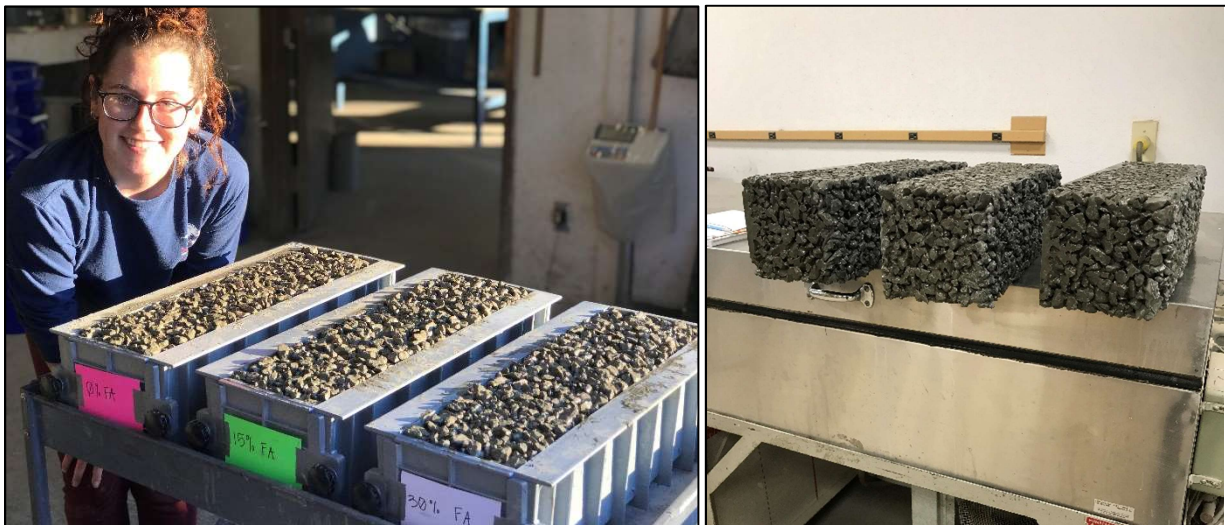
Figure 5. Pervious Concrete Beams for Flexural Strength Testing
