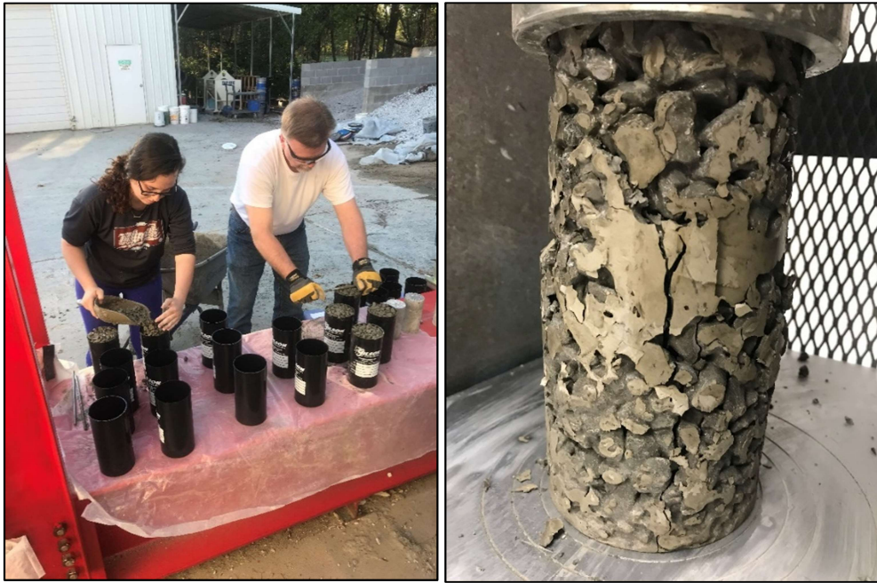
Figure 3. Batching and Testing Pervious Concrete Cylinders
