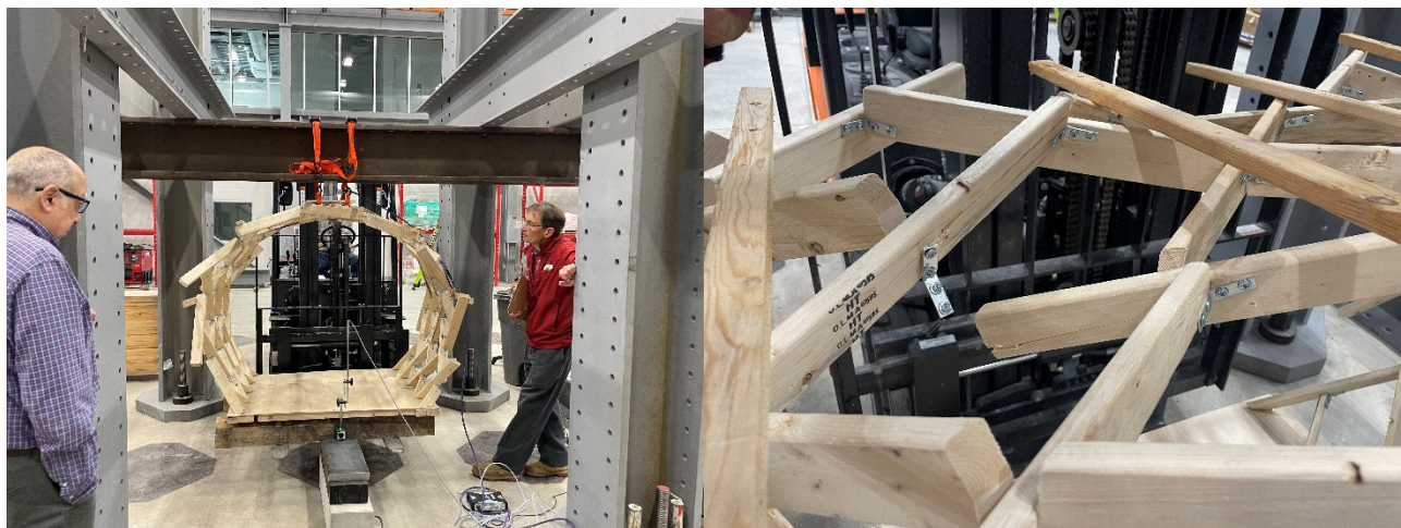
Model during load testing and structural failure points closeup
