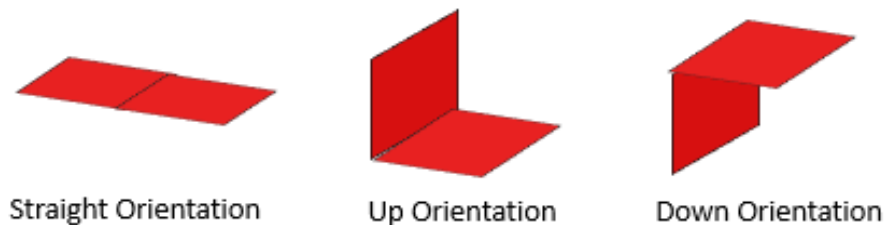
Figure 1: The three different orientations a flexible bond can be in: straight, up, or down.
