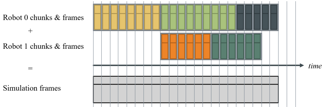
Figure 3-15. Visualization of chunk frames being joined into simulation frames. The gray vertical lines separate frames. The colored rectangles represent the data in each chunk frame. The joining of multiple chunk frames into a single simulation frame is not finely visualized here.
