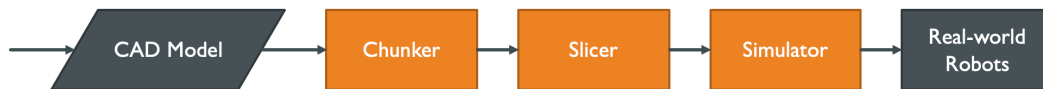
Figure 1-3. Cooperative 3D printing high-level process overview. This thesis is concerned with the processes labelled with an orange color.
