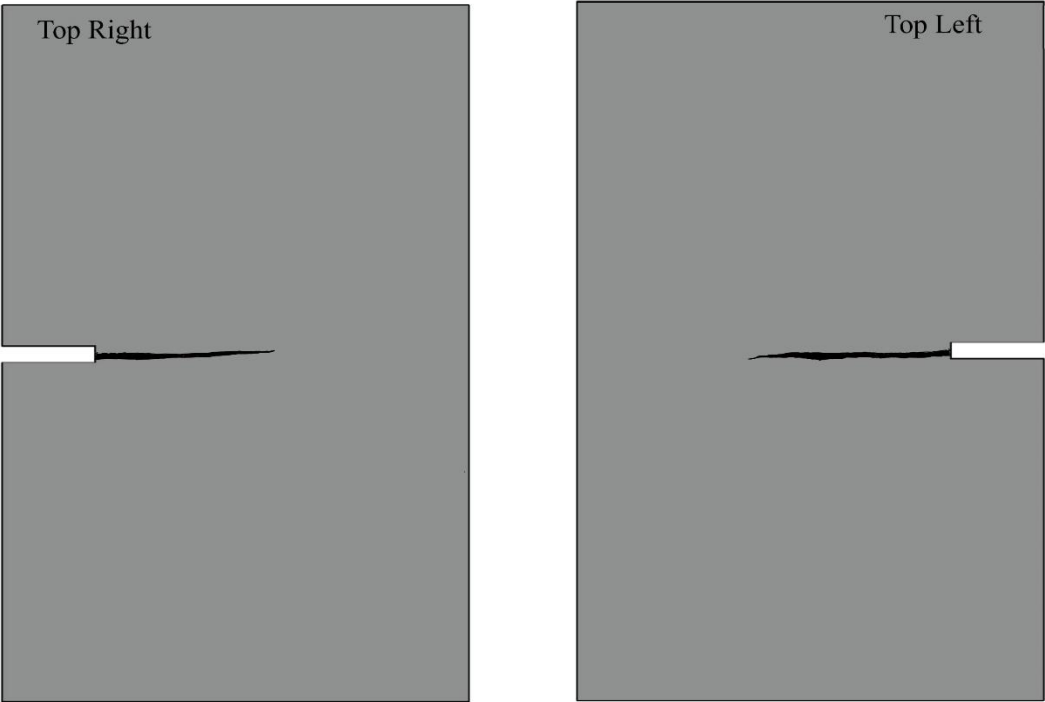
Figure 4. Crack Geometries of Plates after Axial Loading Test
