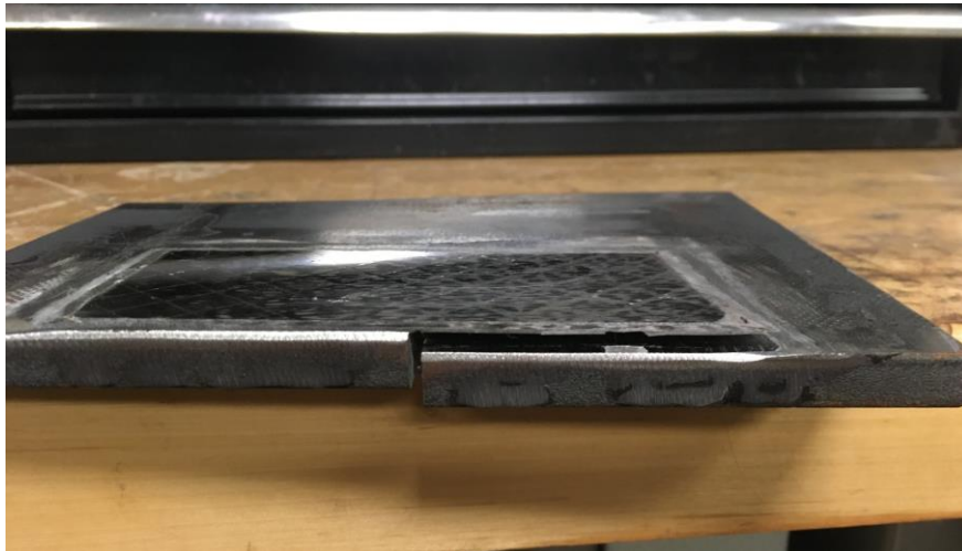
Figure 10. A Steel Plate with CFRP Retrofit After Combined Axial-Torsional Test
