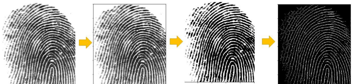
Figure 3. template preprocessing stages represented from left to right where the first image represent the original template and the other represents the stage of making sure is only black and white, improve contrast and transform to a skeletonize image. Fingerprint template extracted from FVC 2004 [12]
