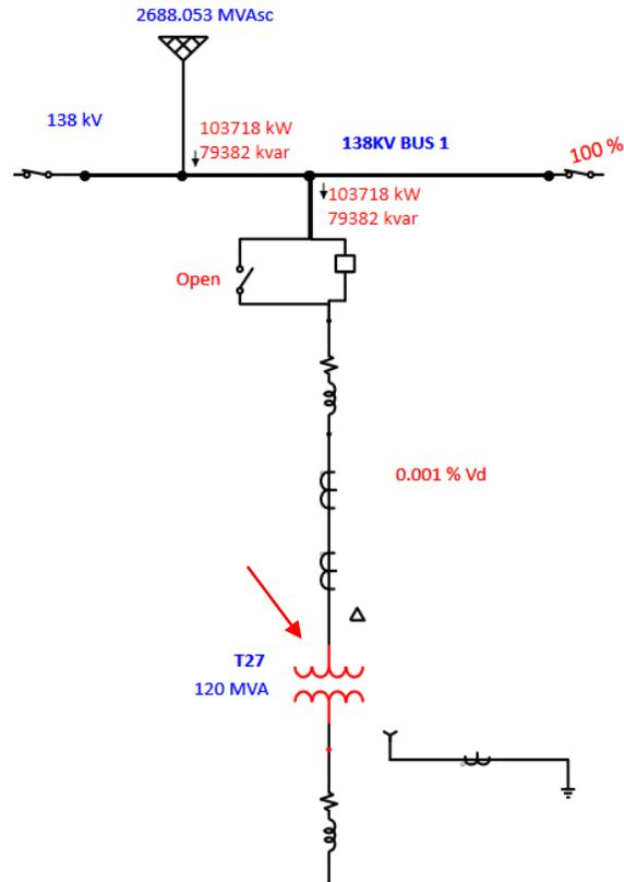
Fig. 4. Load Flow Simulation for Unchanged Conditions.
