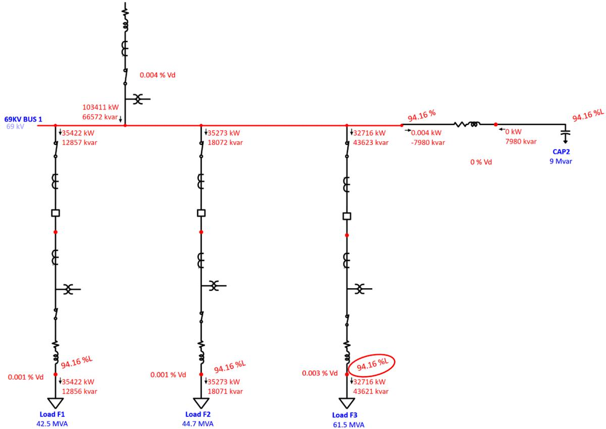
Fig. 3. Load Flow Simulation for Unchanged Conditions.
