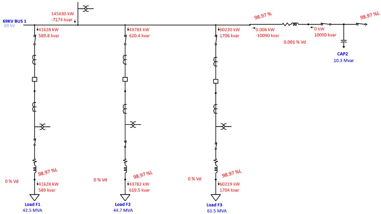
Fig. 12. Installation of Switched Capacitor Bank (Closed Switch).
