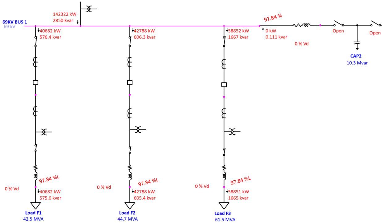
Fig. 11. Installation of Switched Capacitor Bank (Open Switch).
