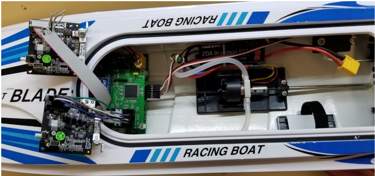
Figure 5: Boat control system installed inside of boat.
