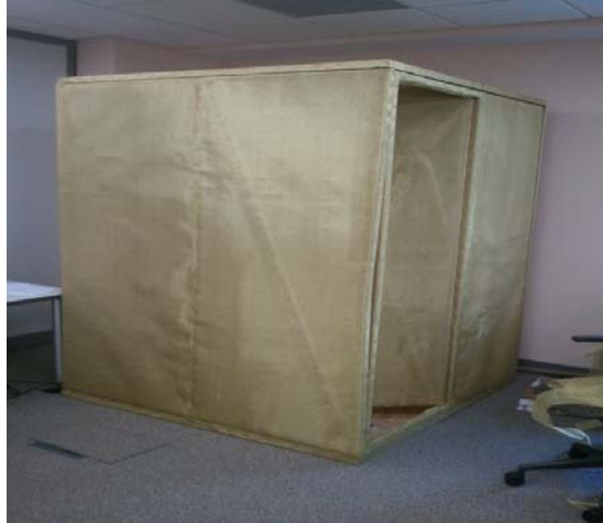
Figure 5: Faraday cage used in experimentation
