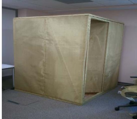
**Figure 5:** Faraday cage used in experimentation
