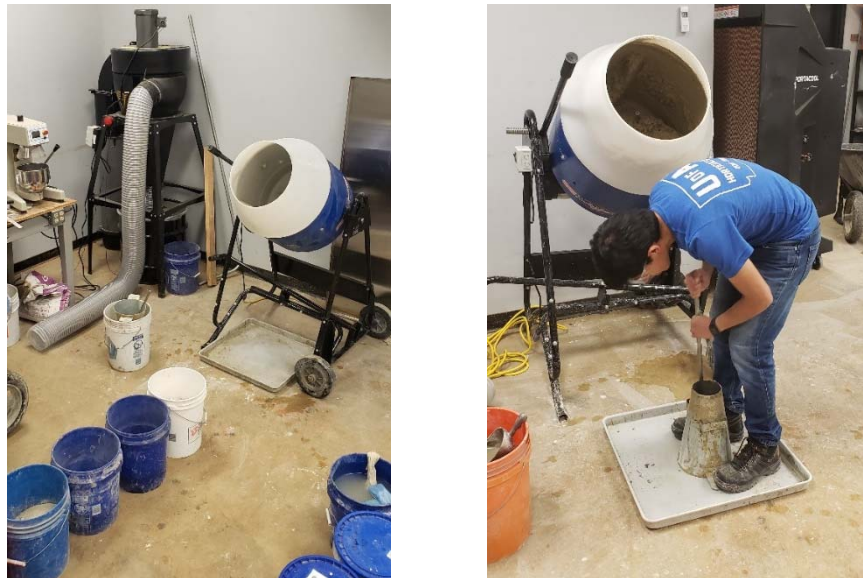
Figure 2a,b. Mixing setup and slump test being performed by graduate student (Photos taken by author)
