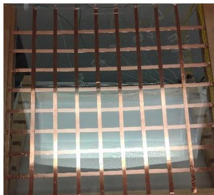
*Figure 6: Capacitive sensor array with 64 sensors*
