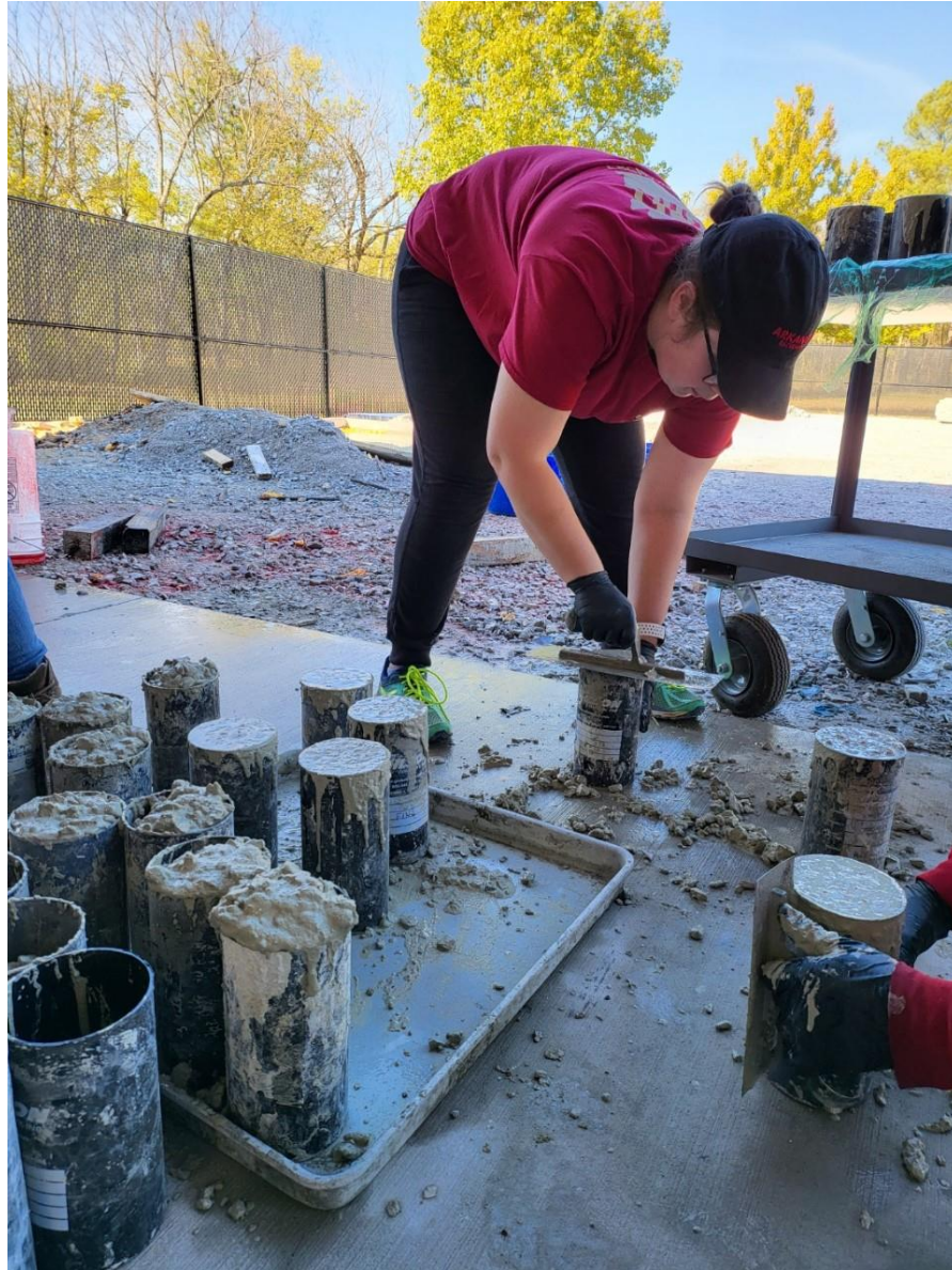
Figure 02. Primary researcher preparing BCSA concrete cylinders
