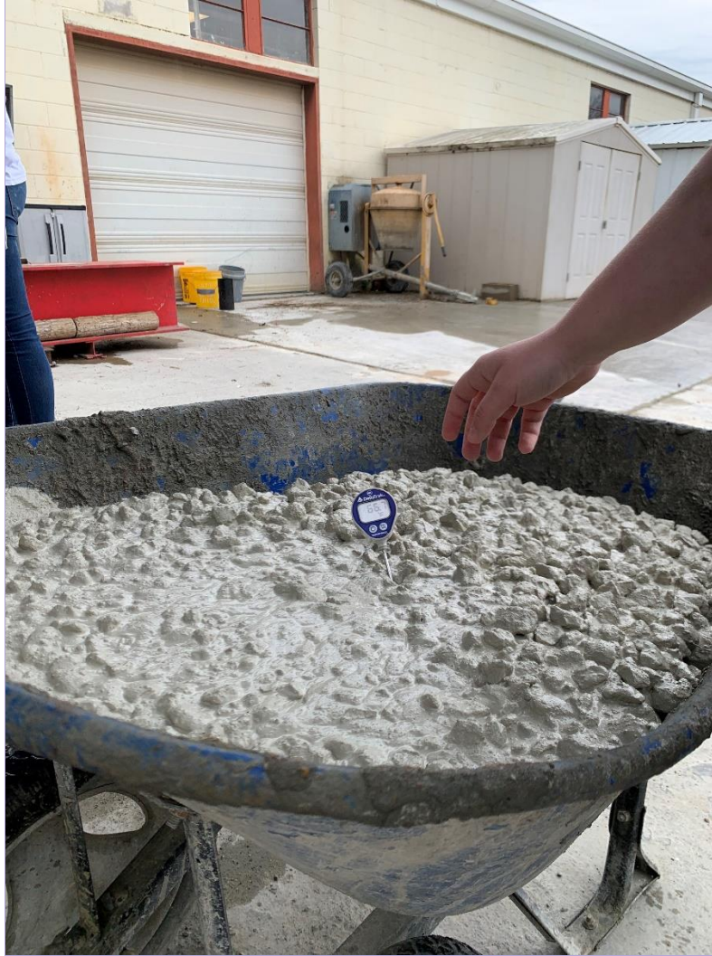
Figure 01. Fresh concrete temperature being measured immediately after mixing
