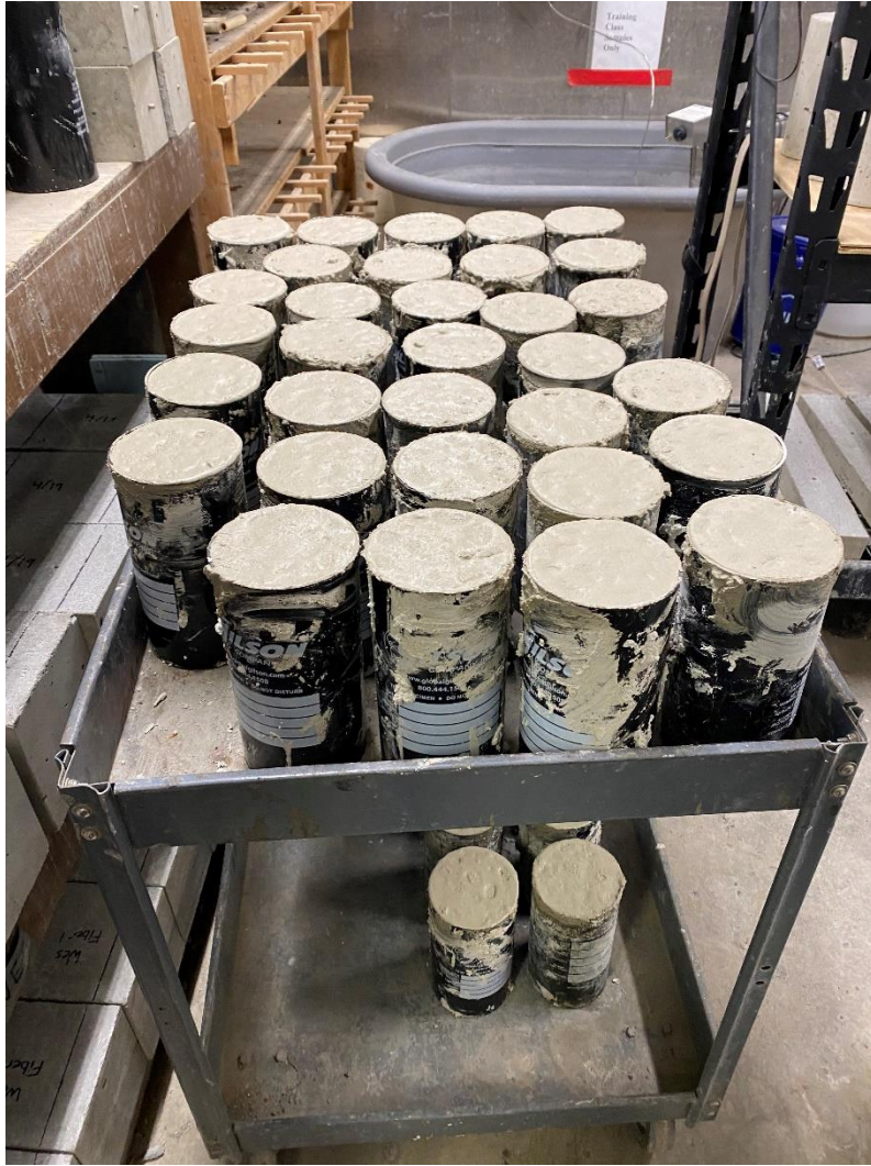
Figure 03. 48 BCSA concrete cement cylinders (Batch 1) in molds before placed in respective curing conditions
