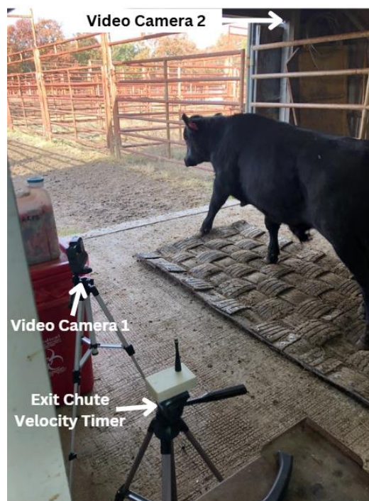
Figure 1. Video camera and exit velocity timer set up to record cattle chute behavior.
