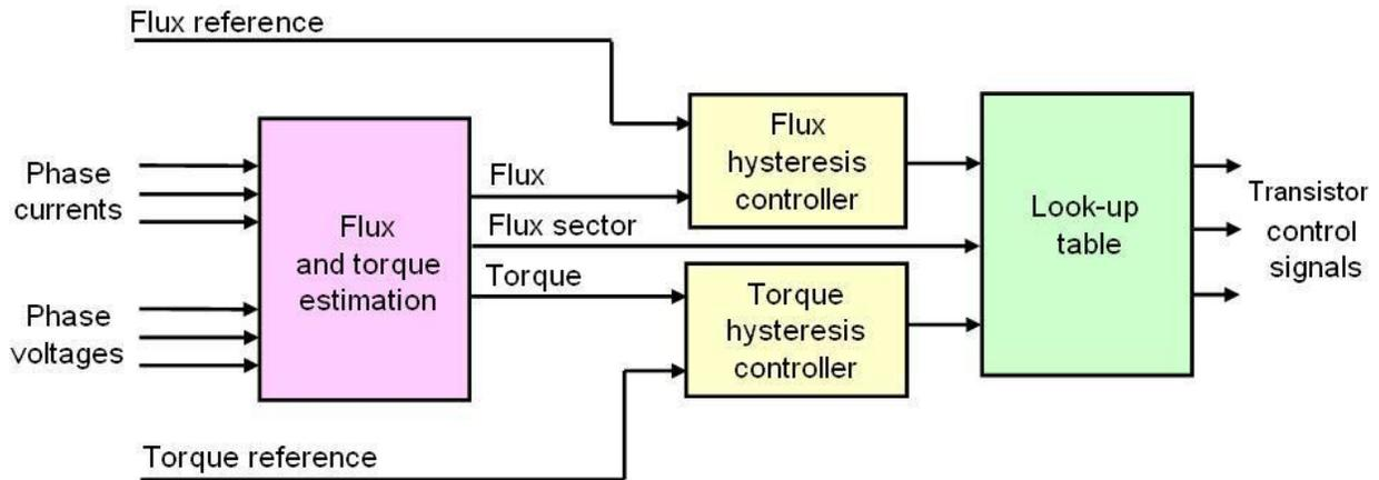
*Figure 1: Operation of DTC Control Method [7]*
