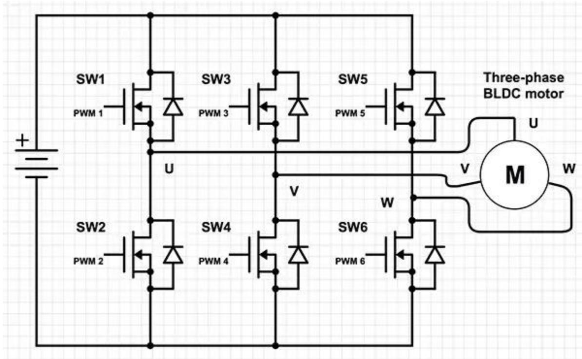
Figure 2: 3-Phase Inverter that Controls Motor [8]
