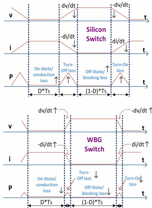
Figure 4: Comparison between WBG and Si Devices
