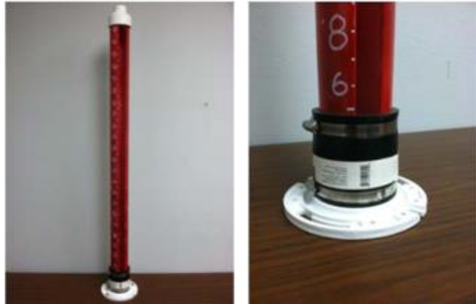
Figure 1. Stiffness Raveling Mechanism (Hill & Braham, 2016)
