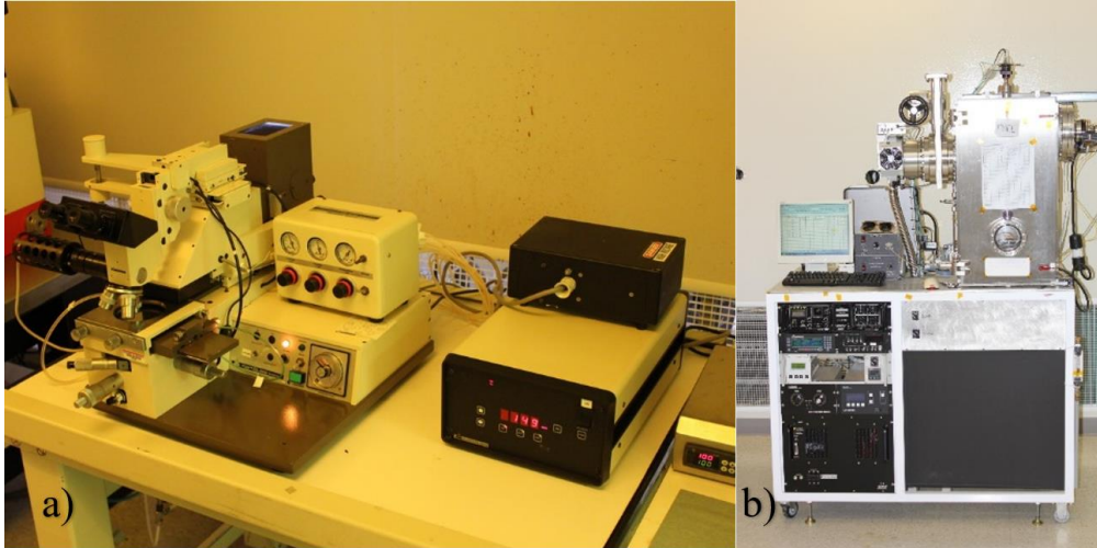
Figure 7. Cleanroom and Metallization Equipment a) Suss Microtec MJB3 contact aligner. b) Specialty Vacuum Tech. PVD-1 E-Beam evaporator. Used with permission by Syam Madhusoodhanan.
