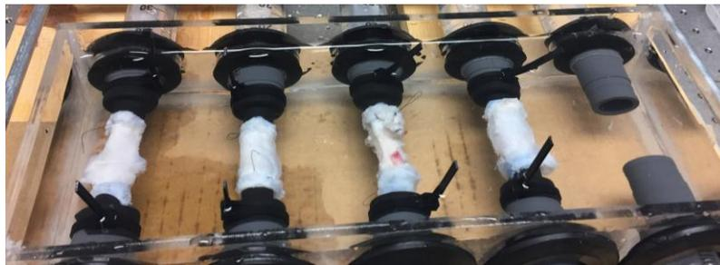
*Figure 3. Four valves were placed in the fatigue apparatus for ten hours for the preliminary mechanics testing. The vein segments are attached to the PVC connectors using zip ties.*
