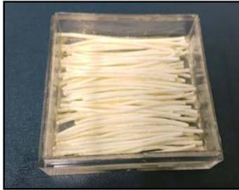
**Figure 2** Hollow fiber membrane diffusion chamber for evapoporometry.
