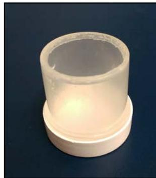
**Figure 1** Flat sheet membrane diffusion chamber for evaporometry.
