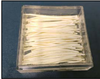
Figure 2 Hollow fiber membrane diffusion chamber for evapoporometry.
