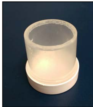
Figure 1 Flat sheet membrane diffusion chamber for evaporometry.
