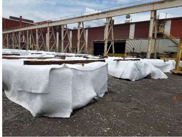
FIGURE 6: Steel Bars Slow Cooling under a Blanket
