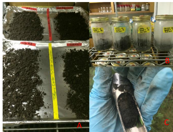
Figure 2: A) Dry treatment. B) Moist treatment. C) Soil sample collection.
