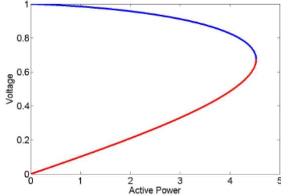
**Figure 1.** Example of a P-V curve of an electrical system, given to illustrate the regions of stability of a power system [4]
