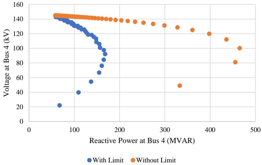
Figure 9. Q-V curve of system intact simulations
