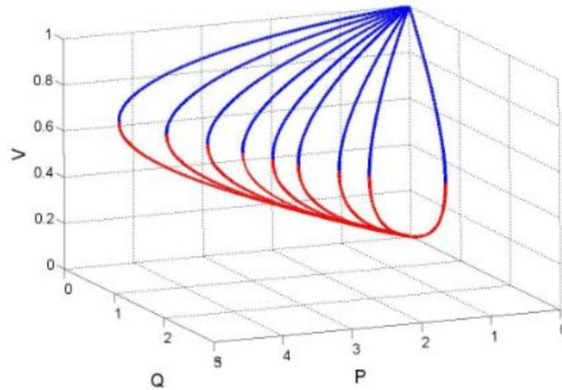
**Figure 2.** Example of several P-V curves where reactive power Q is also altered [4]
