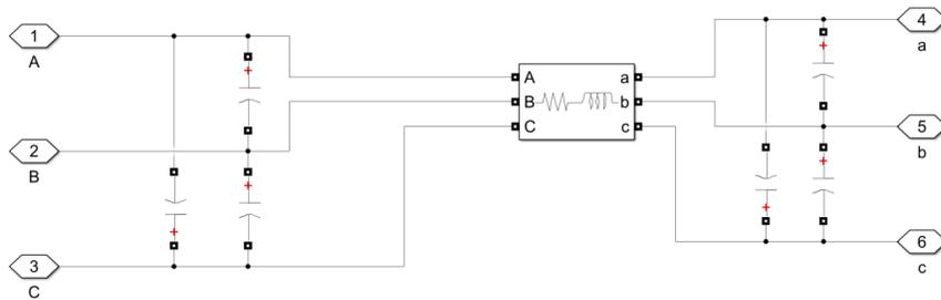
**Figure 6. Modified PI design for modeling transmission lines**
