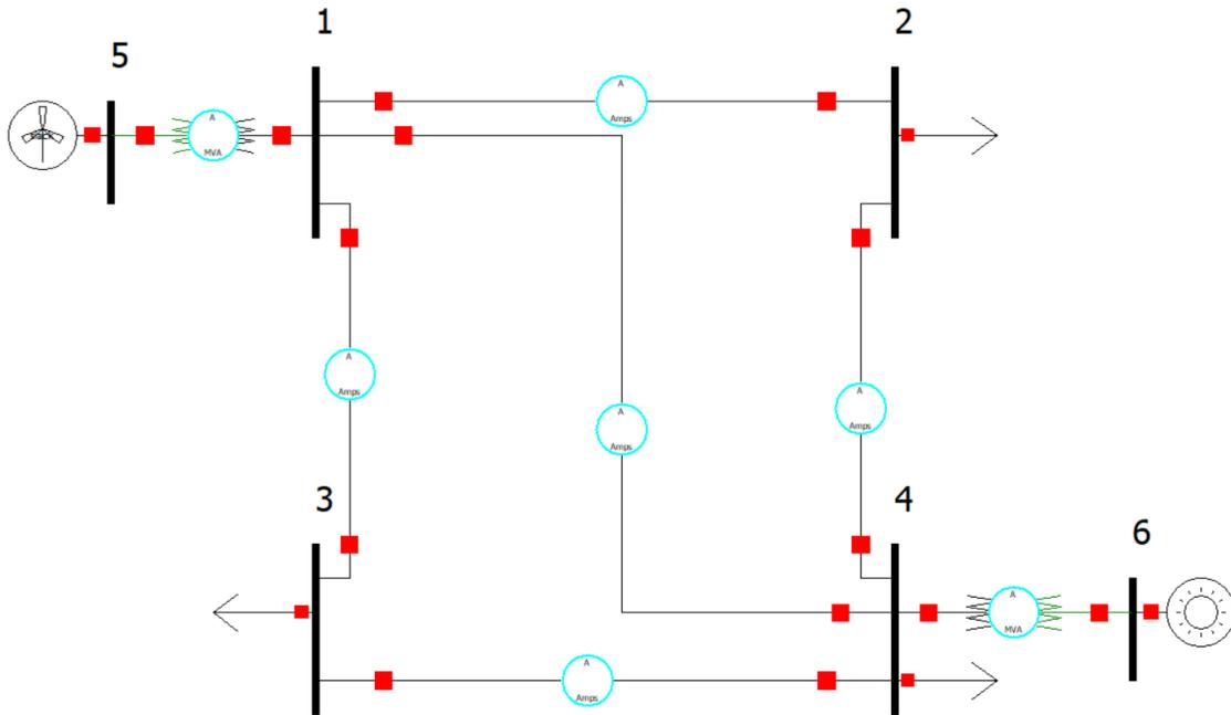
**Figure 3.** 6-bus weak grid IBR system used for testing
