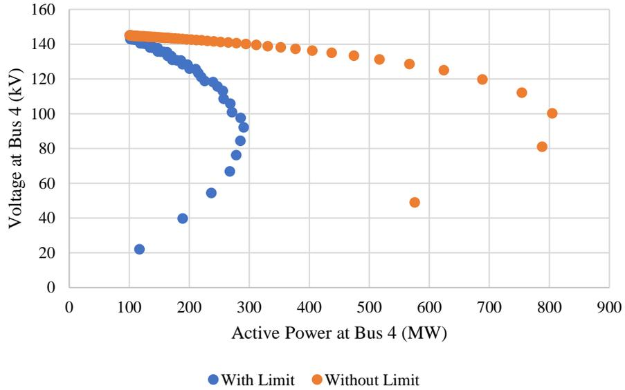
Figure 8. P-V curve of system intact simulations
