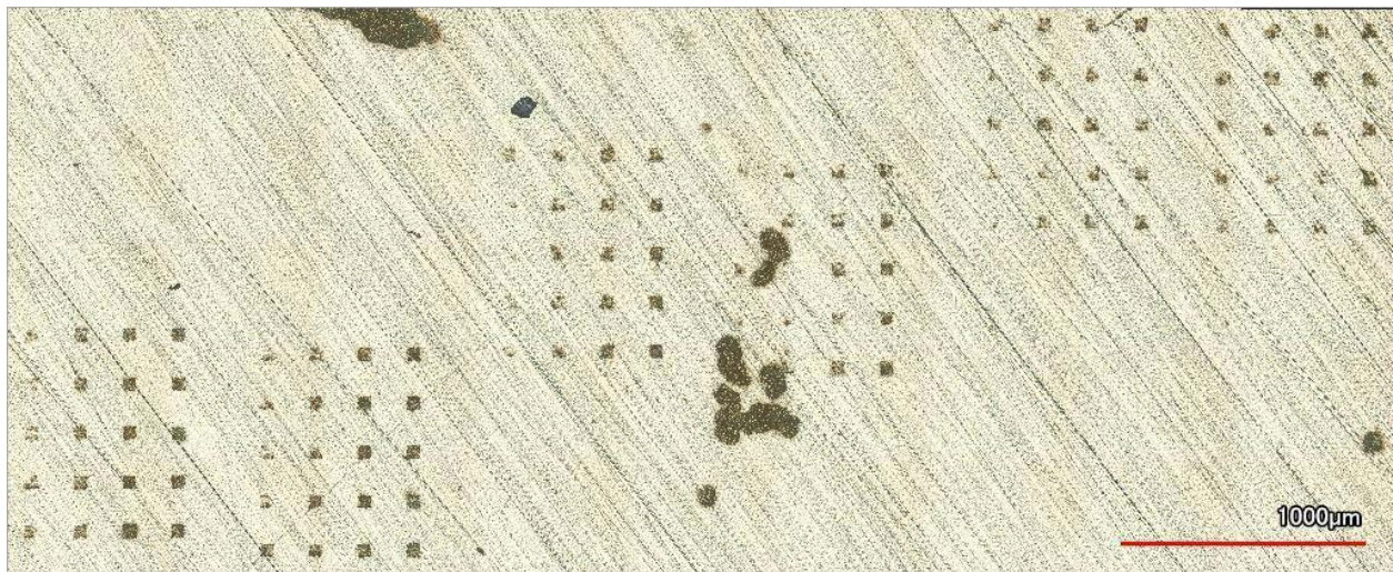
Figure 4: Optimization tests for printing parameters. Bottom left are two arrays for 1 \mu\text{m} slicing and 0.5 \mu\text{m} hatching distance. Middle two arrays represent the 1.25 \mu\text{m} slicing distance with a 0.75 \mu\text{m} hatching distance. Top right two arrays are for the 1.5 \mu\text{m} slice and a 1.0 \mu\text{m} hatching distance.
