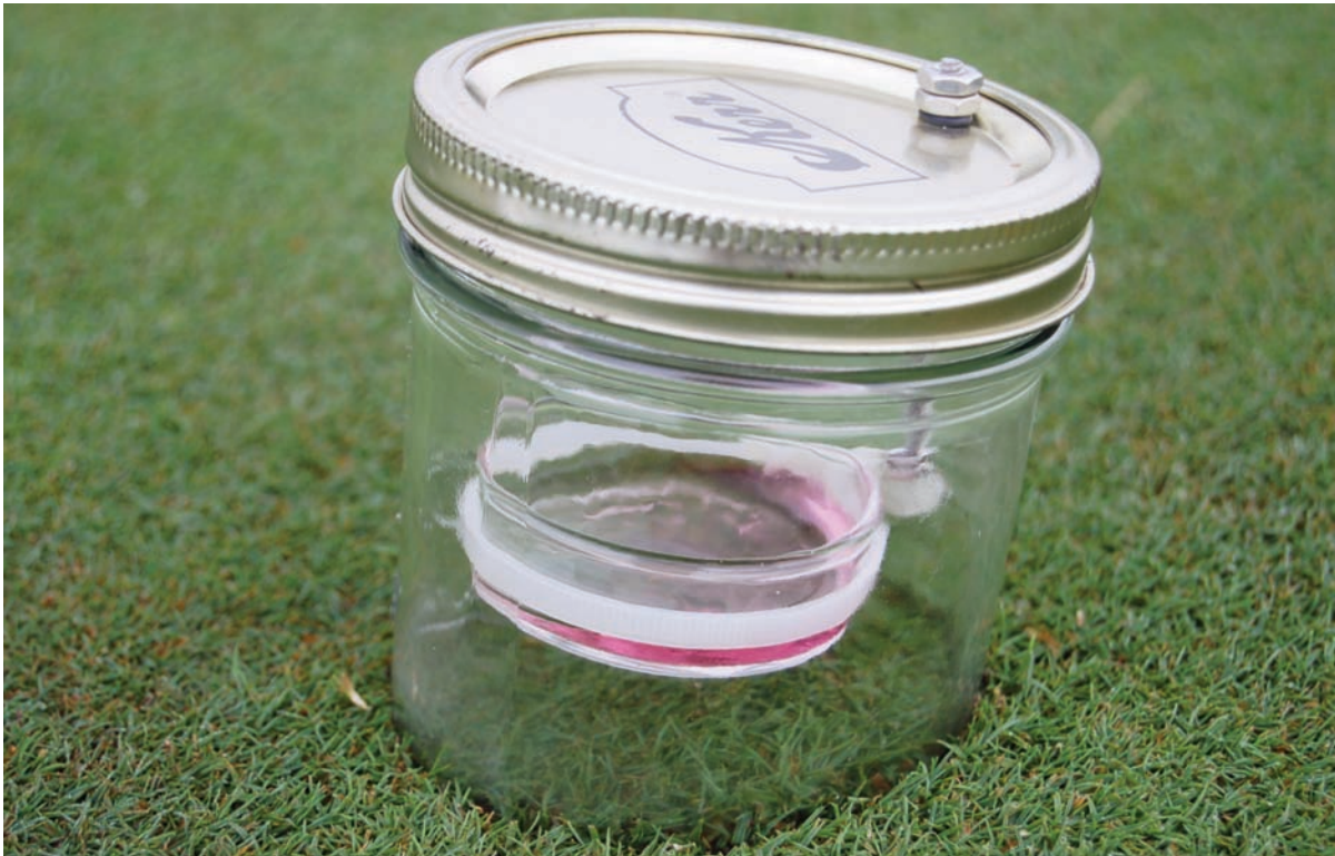
Fig. 1. Apparatus used for in-field ammonia volatilization estimates.
