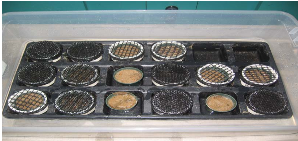
Fig. 2. Various intensities of shade cloth were stretched over the top of PVC rings and cinched tightly to the outside of the ring with plastic fasteners. These were then placed over the pots containing soil and bermudagrass seed.
