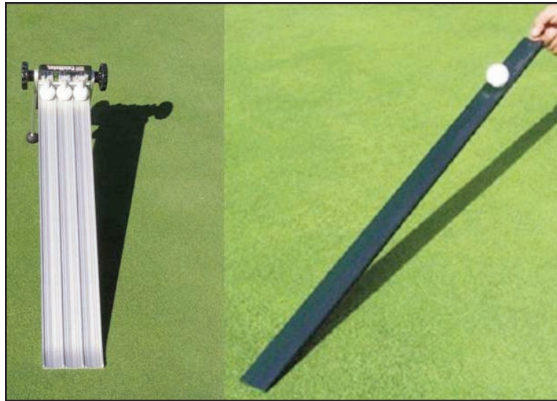
Devices used for measuring putting green speed. Pelzmeter (left) and Stimpmeter (right).
