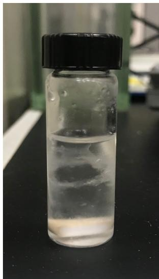
**Figure 6.** PF127 and PVA hydrogel with visible clump
