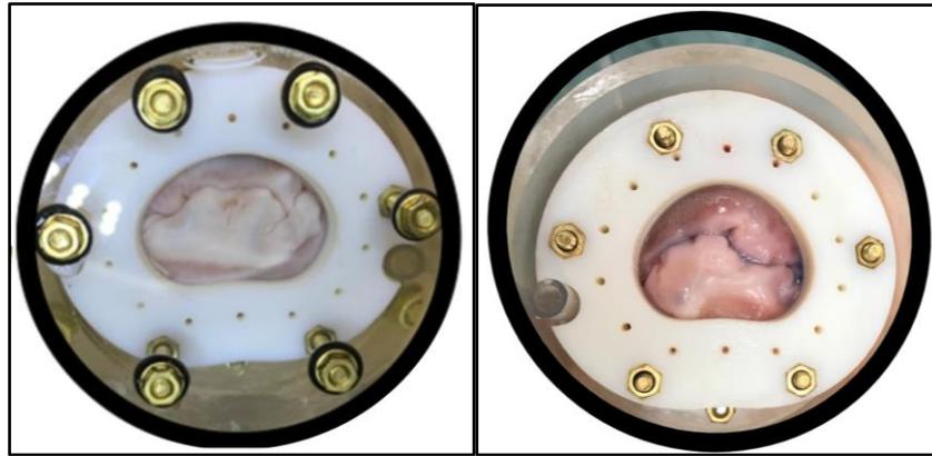
**Figure 5A.** MV leaflet closure for MRI using fluid pressure (5). **Figure 5B:** MV leaflet closure using air pressure with Vetbond adhesive for  $\mu$ CT.
