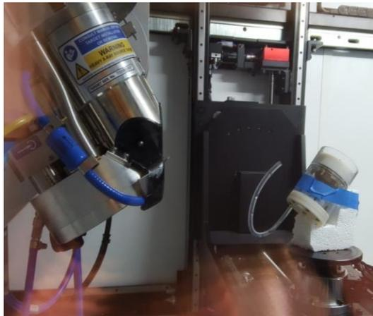
**Figure 4.** Mounted mitral valve is imaged using Micro CT at 45°
