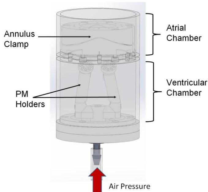
**Figure 2.** Mitral valve imaging apparatus (6).
