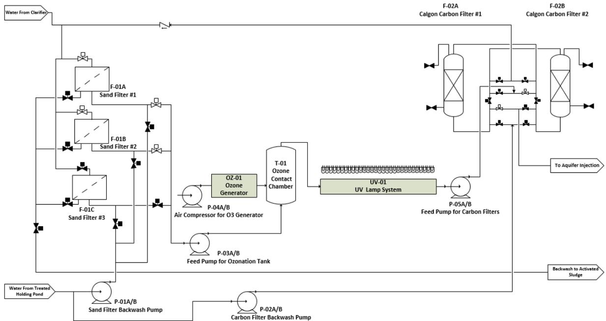
Figure 6: Process flow diagram for industrial scale system
