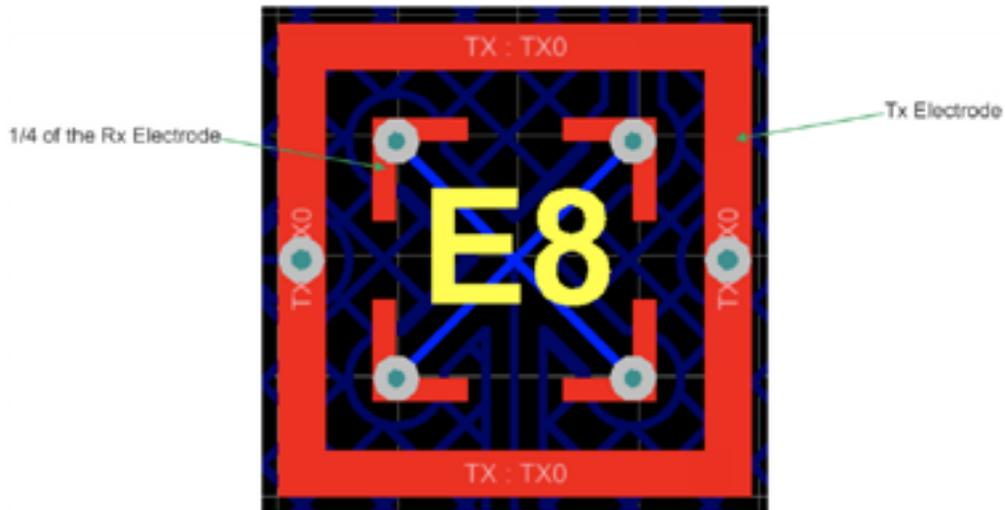
Figure 3: Design of Mutual Capacitance Sensor [14]
