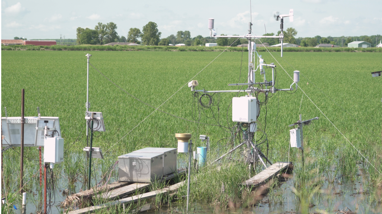
Figure 2: Eddy covariance system in Stuttgart, AR rice research field used to measure GHG concentrations
