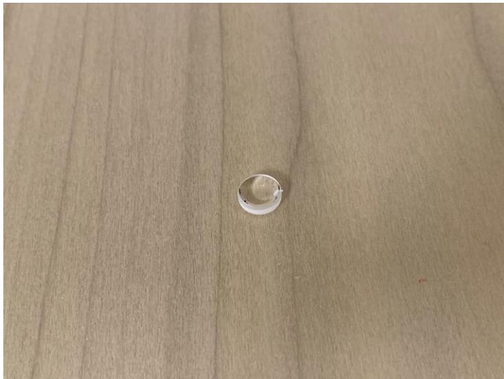
*Figure 4. Collimator Lens (FL = 30 mm) (7)*
