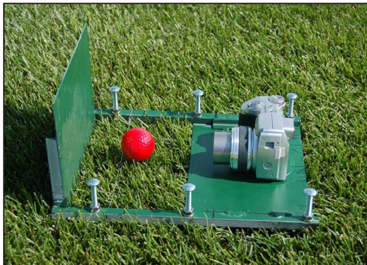
Fig. 1. Device used to collect images of a golf ball resting in the turf and later analyzed using digital image analysis.
