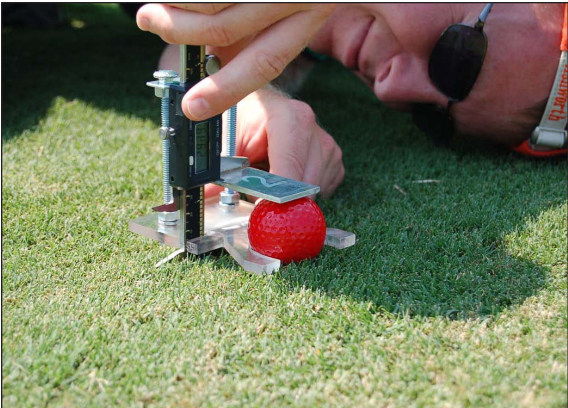
Fig. 2. The Lie-N-Eye II, a device developed by the University of Illinois to measure the height of a golf ball above the canopy.
