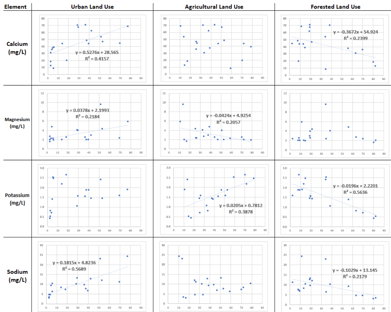
Figure 3: Relationships between the Macro-Elements Calcium, Magnesium, Potassium, and Sodium, and Varying Land Uses in the Stream's Watershed (Based On 2012 Land Use Land Cover, modelmywatershed.org)
