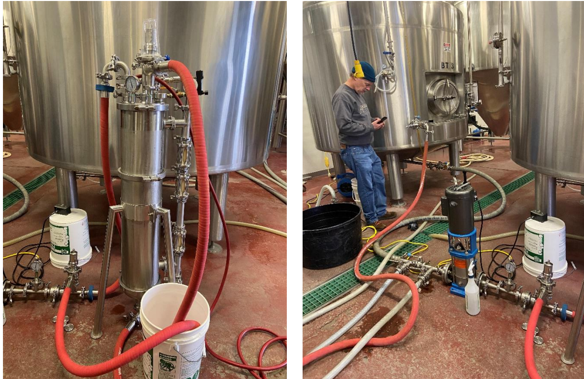
Figure 4: Using the Carbo Rock-It to carbonate a production batch of IPA
