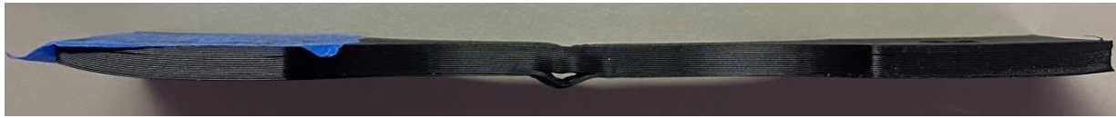
Figure 8. Linear infill pattern with 20% infill density sample after 50 bends, bottom view
