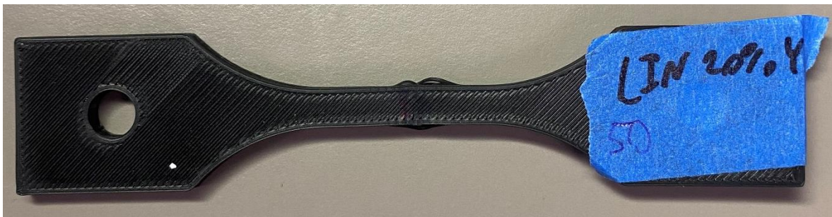
Figure 6. Linear infill pattern with 20% infill density sample after 25 bends, side view
