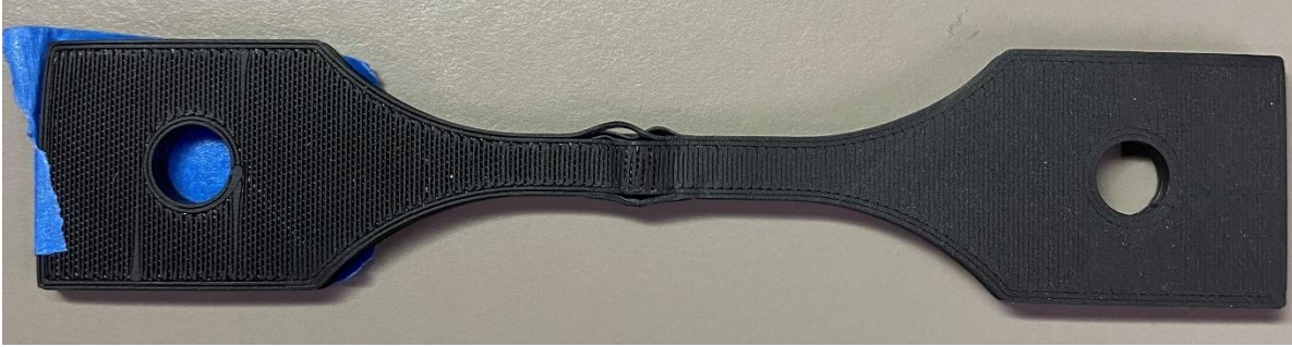
Figure 8. Linear infill pattern with 20% infill density sample after 50 bends, bottom view
