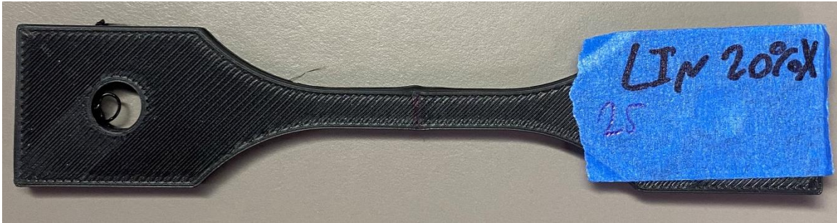
Figure 4. Linear infill pattern with 20% infill density sample after 25 bends, top view
