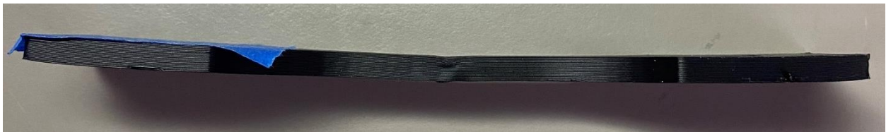
Figure 5. Linear infill pattern with 20% infill density sample after 25 bends, bottom view
