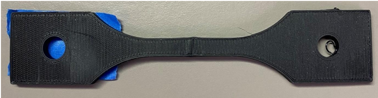
Figure 4. Linear infill pattern with 20% infill density sample after 25 bends, top view
