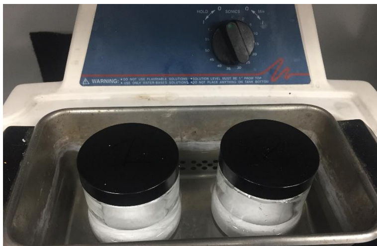
Figure 6. Sonication of Sorbitol solution.
