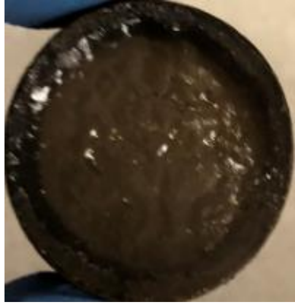
Figure 12. Graphene oxide sample with strong dispersion (GA-L).
