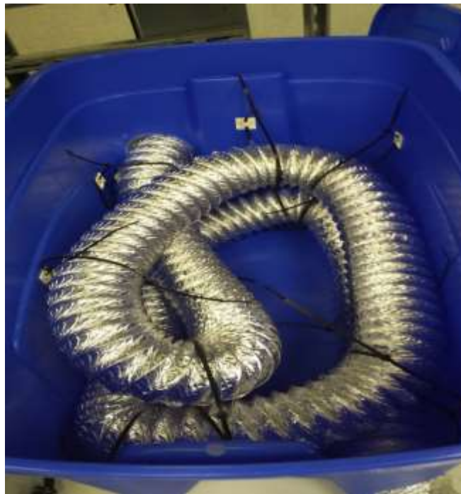
Figure 13 : Cooler construction with 20' duct
