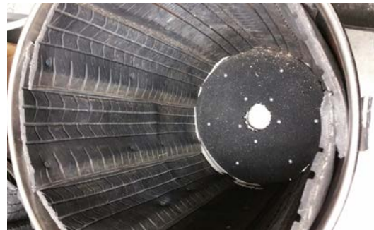
Figure 7. Treads Inside Ball Mill
