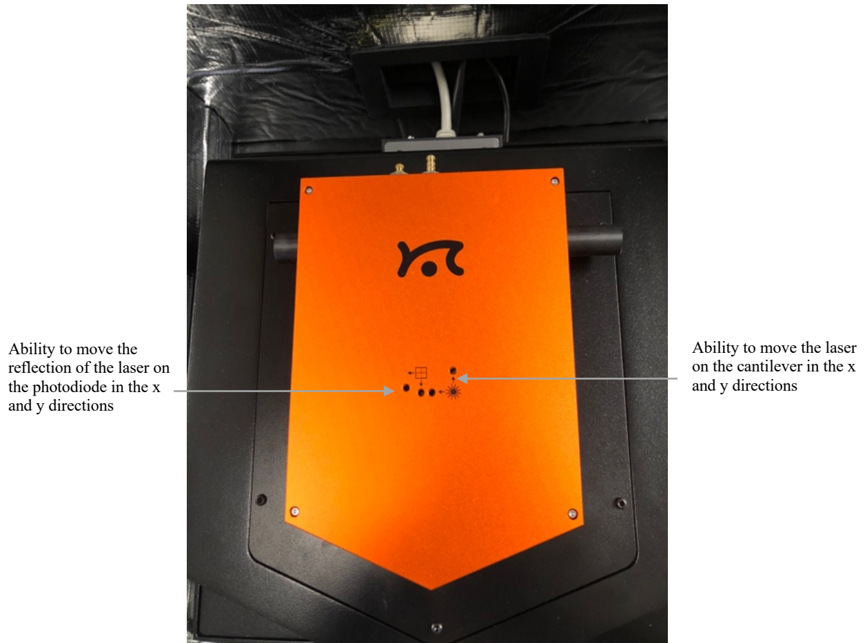
Figure 9: Screw holes that allowed the laser to move its direction on the cantilever and its reflection on the photodiode in the x and y directions.
