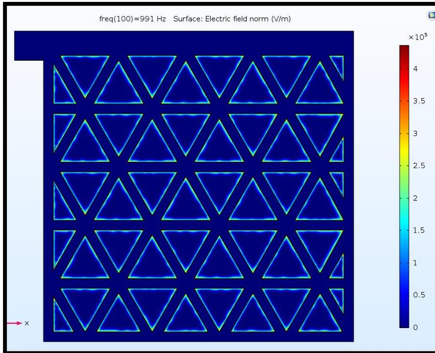
Figure 14: Electric Field Concentration on Triangle DBD
