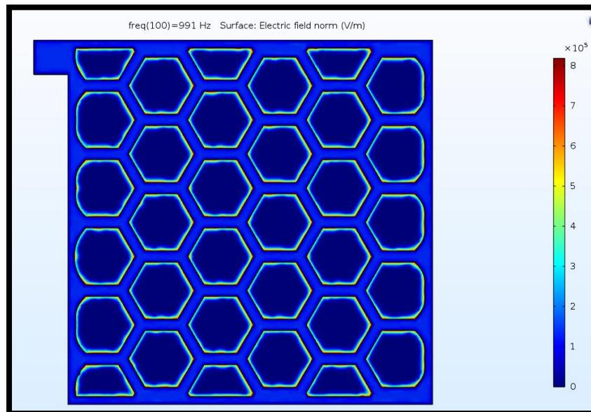
*Figure 13: Electric Field Concentration on Hexagonal DBD*
