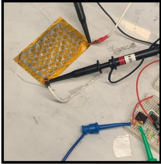
*Figure 2: Plasma Actuation Test Setup*
