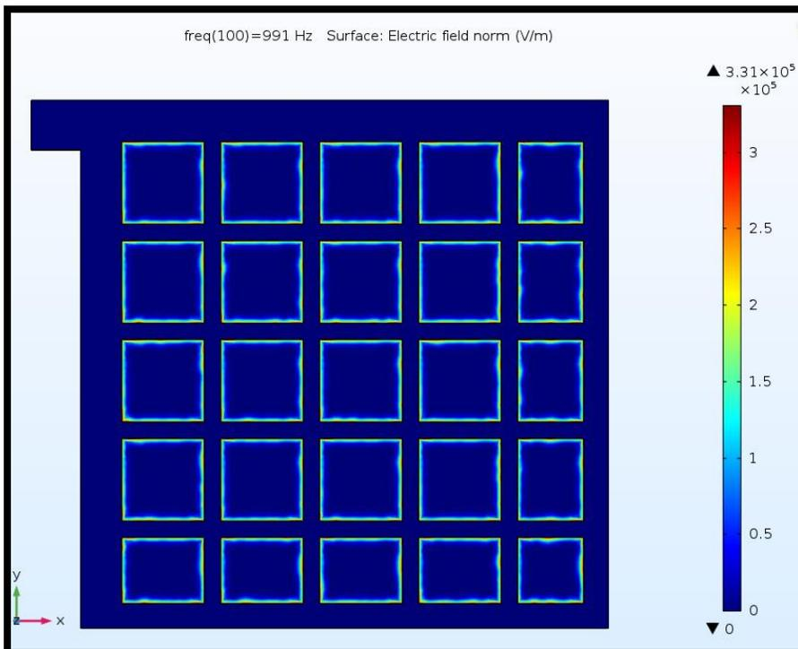
Figure 15: Electric Field Concentration on Square DBD
